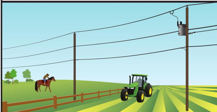
Vertical Clearance at Largest Vertical Sag Table 232-1
