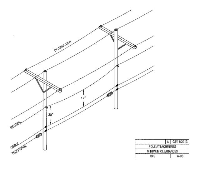
Drawing A-07-Minimum Clearance at Pole/Midspan from Secondary
