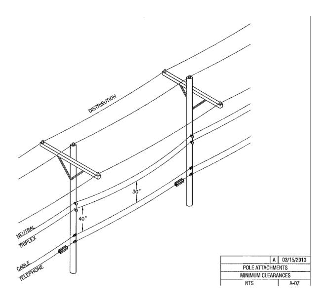
Drawing A-08—Minimum Clearance at Pole/Midspan from Primary
