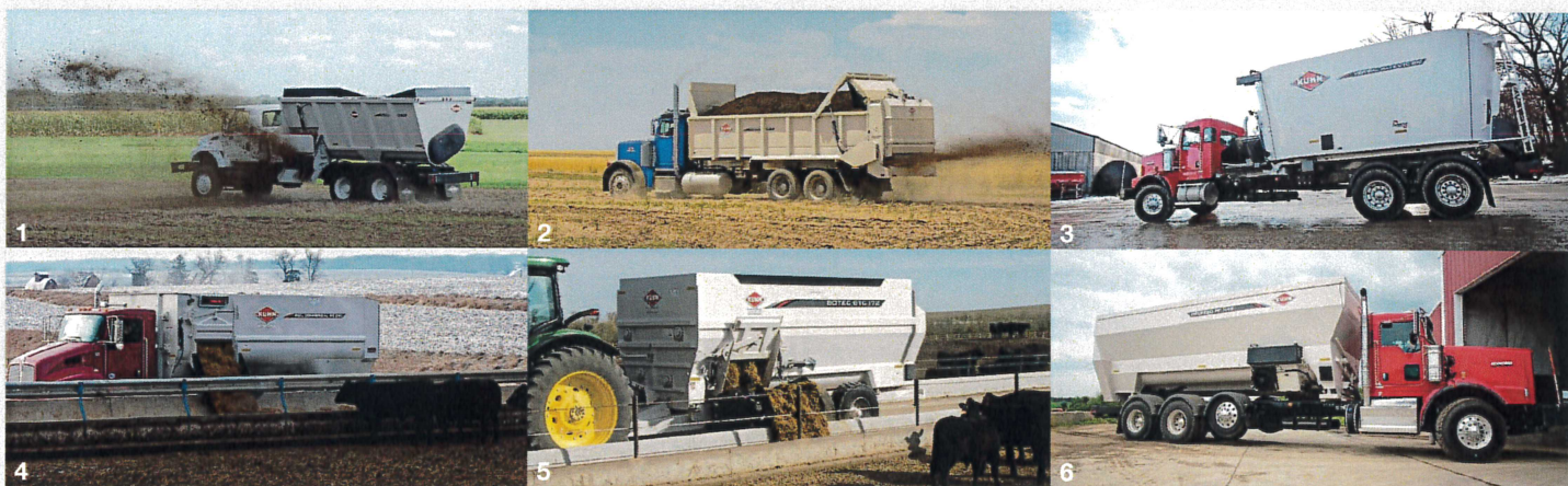
1. Side-Discharge Spreaders – 2. Apron Box Spreaders – 3. Vertical Twin-Auger Mixers – 4. Reel Mixers – 5. 4-Auger Mixers – 6. Delivery Boxes
