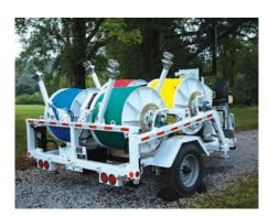
USER-FRIENDLY DRUM ENGAGEMENT COUPLER ALLOWS FOR SAFE AND PRODUCTIVE DRUM ENGAGEMENT DURING PULLING OPERATIONS
